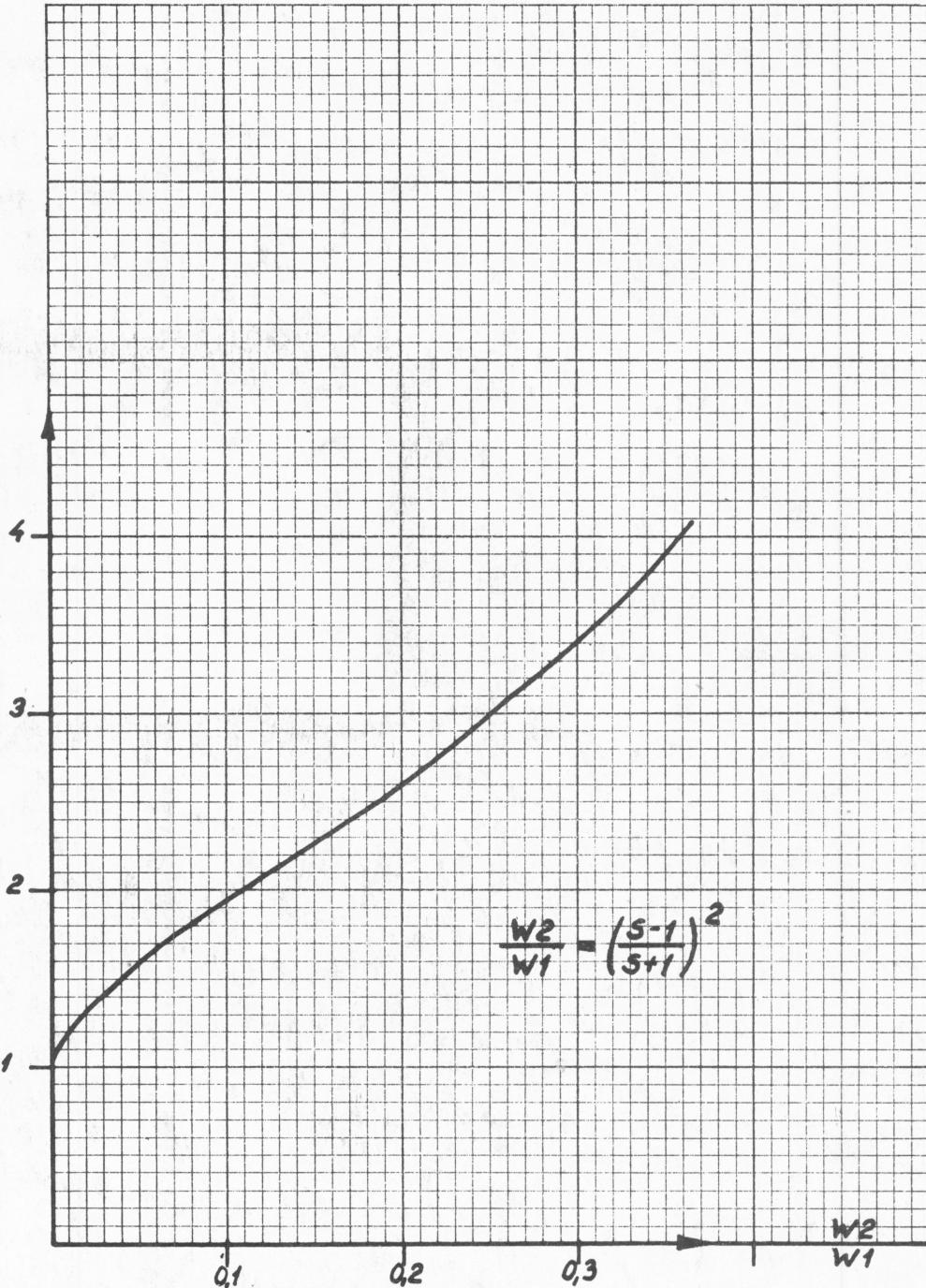
$\frac{W_2}{W_1}$  is the ratio between the reflected and the transmitted power in a transmission line.
